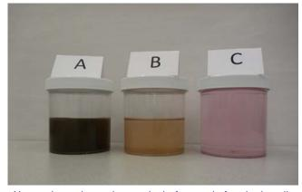
Above photo shows the results before and after the installation of a Spirovent® Air/Dirt Separator by Spirotherm, Inc.
